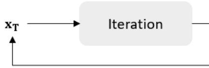
Figure 4.2: Graphic displaying the continuation of state across iterations, \mathbf{x}_1^j = \mathbf{x}_T^{j-1}
