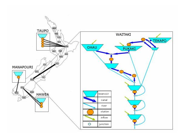
Figure 2: Approximate network representation of New Zealand electricity network showing main hydro-electricity generators
