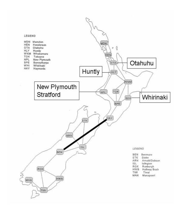
Figure 1: Approximation of New Zealand transmission network showing location of major thermal generators. The bold line represents a HVDC cable connecting the South and North islands.
