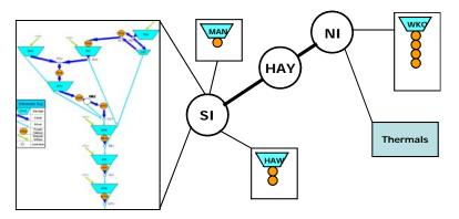
Figure 3: The 3 node transmission network and major generators in DOASA.
