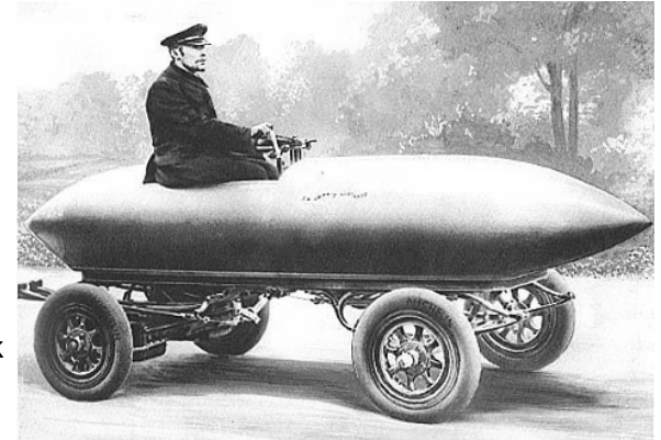
1899, Camille Jenatton reached a speed record of 109 km/h with his cigar-shaped electric car powered with lead-acid batteries.
